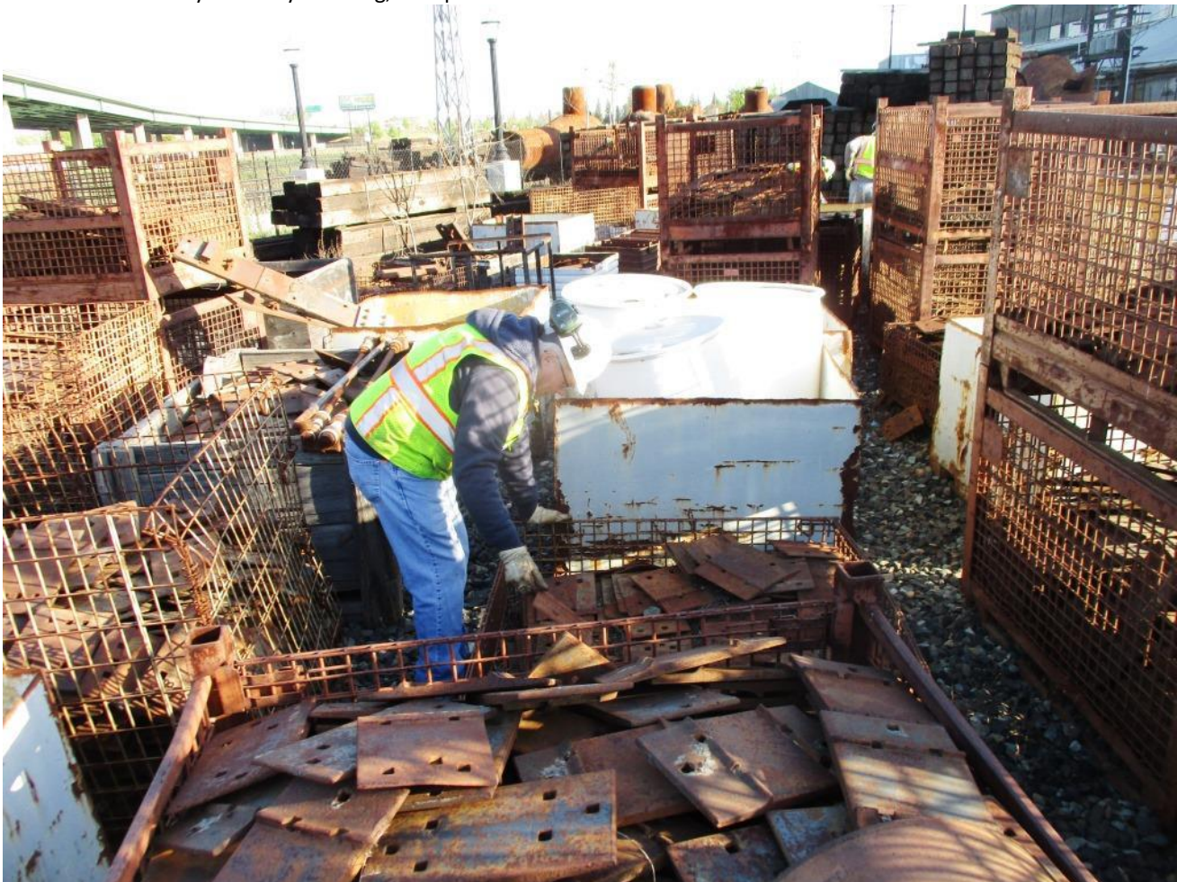
Bill searches for 90-pound tie-plates in the materials yard
